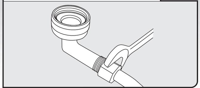
Connect the  $\frac{3}{8}$ " compression fitting to the water supply line prior to installing the unit into the cabinet opening. Attach such that the  $\frac{3}{4}$ " connection is facing upward.
